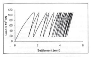
From the load settlement data total and permanent settlement of the footing with the increase in number of load cycles for different cases were obtained. Total and permanent settlement of the footing for unreinforced, reinforced bed and reinforced bed with aging period of 4 months are presented in **Fig. 5**.
