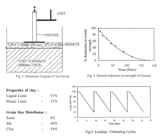
Average cohesion of artificially consolidated soil bed is 21 kN/m<sup>2</sup>. This was determined from vane shear tests. After preparing the soil bed a layer of JGT was placed over it. Over this a 50mm thick compacted sand bed was laid.
