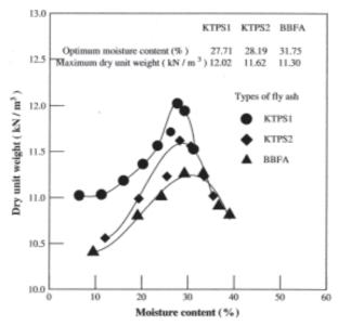
Fig. 2 : Dry unit weight versus moisture content curves.
