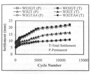
Fig. 5 Increase in Settlement with Aging under various Load Cycle
