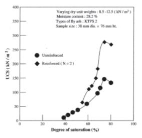
Fig. 5 : UCS versus degree of saturation curves with varying dry unit weights.
