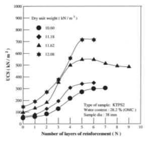
Fig. 7 : UCS versus number of layers of reinforcement (N) for different dry unit weights of fly ash
