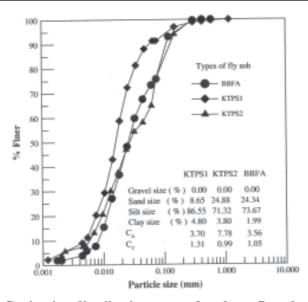
Fig. 1. Grain size distribution curve for three fly ash samples.
