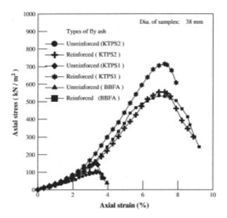
Fig. 4. Typical axial stress versus axial strain curves for unreinforced and reinforced fly ash.
