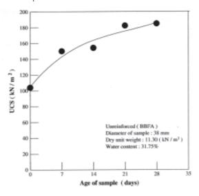
Fig. 10 : UCS versus age of samples of fly ash
