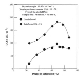
Fig. 6. UCS versus degree of saturation curves with varying moisture contents.
