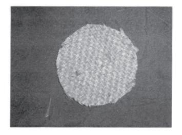
Fig. 3. Photograph of jute geotextile fabric.
