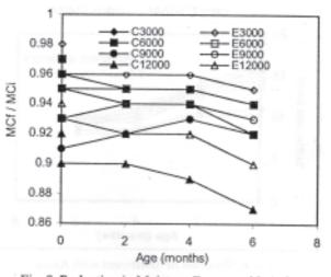
Fig. 8 Reduction in Moisture Content with Aging
