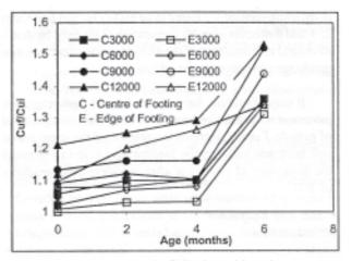
Fig. 7 Increase in Cohesion with Aging
