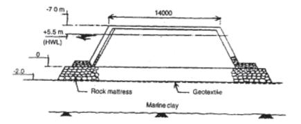
Figure 6 : Geotextile in guide bound in soft marine clay at Nava-Seva Port.
