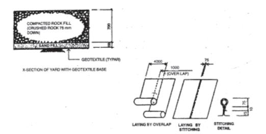
Figure 2 : Geotextile in fabrication yard near Haldia Port.
