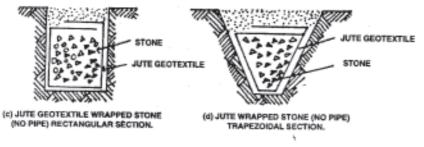
Figure 12 : Jute Geotextile in trench drains
