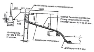
Figure 7 : Geotextile below revetment for river bank erosion in Lakwa, Assam
