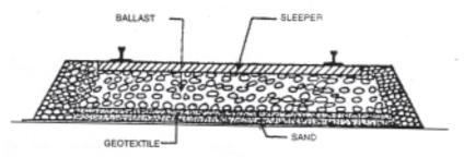
Figure 5 : Geotextile in strengthening railway track.
