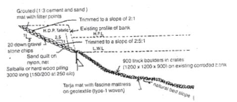
Figure 8. Geotextile in erosion control at Farakka.
