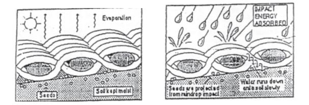
Fig. 1 : HARMLESS SURFACE DRAINAGE (After Rankilor, 1994)
