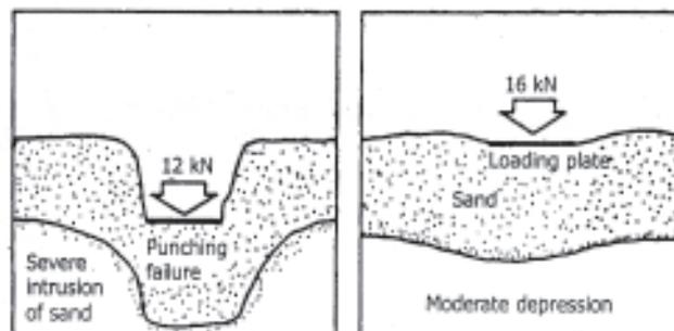
Figure 4 : Subgrade/Subbase Interface Profile with and without Jute Fabric under Different Static Loading
