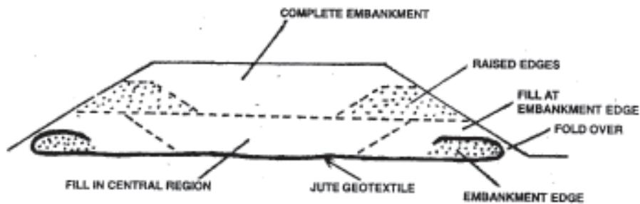
**Figure 11 : Geojute in embankment construction**
