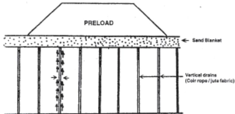
**Figure 13 : Geojute in vertical drainage**
