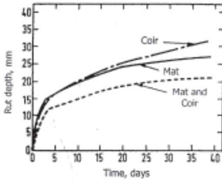
Figure 8 : Rut Depth-Time Relationship for Sustained Loading Test
