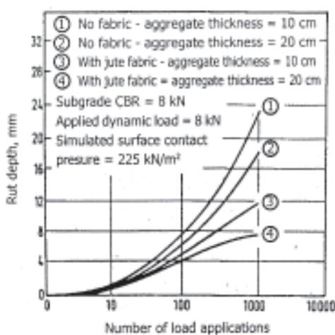
Figure 1 : Typical Surface Rut Depth Vs Number of Load Applications Plots for Dynamic Load Test using Jute Fabric alone
