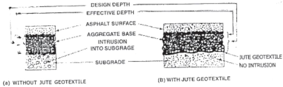
**Figure 9 : Pavement with Jute Geotextile**
