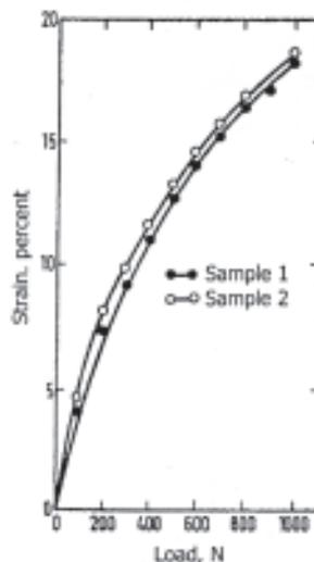
Figure 6 : Stress-strain Behaviour of Coir Strand
