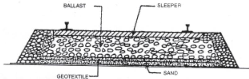
**Figure 5 : Geotextile in strengthening railway track.**
