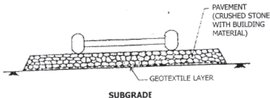
**Figure 1 : Geotextile in temporary roads.**
