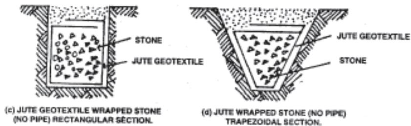
**Figure 12 : Jute Geotextile in trench drains**
