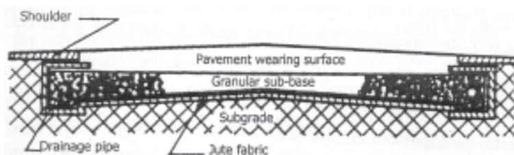
Figure 12 : Position of Jute Fabric in Road Structure
