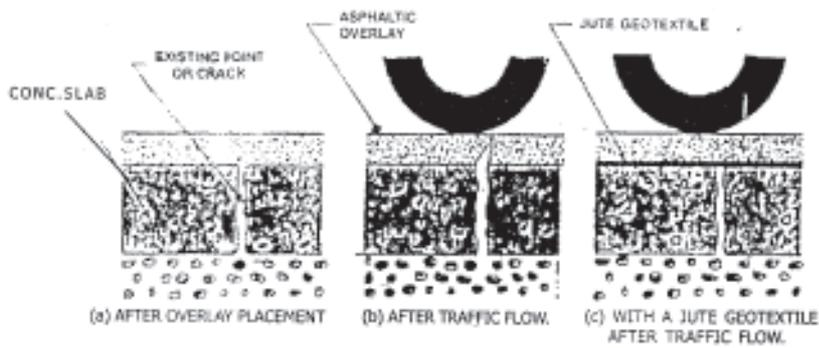
**Figure 10 : Control of reflective cracking with Jute Geotextile**
