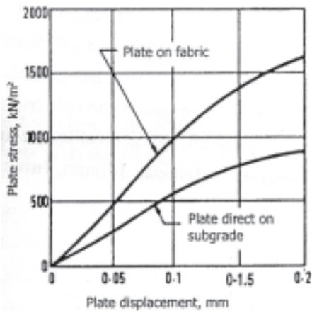
Figure 11 : Effect of Jute Fabric on Bearing Capacity of Subgrade Soil
