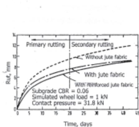
Figure 5 : Rut-Time Relationship for Sustained Seven Weeks Loading Test
