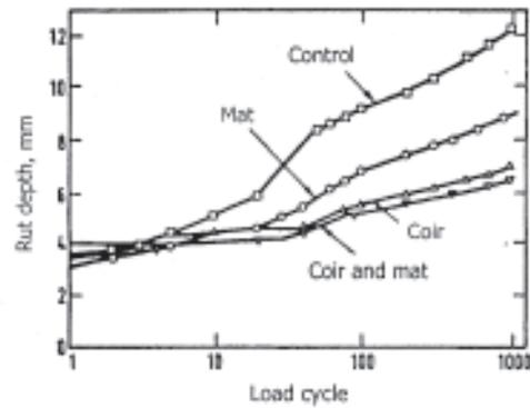
Figure 9 : Rut Depth Vs Number of Load Application
