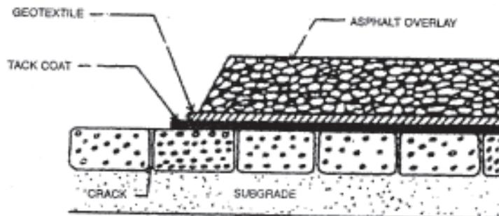
Figure 4. Geotextile as pavement overlay for treatment of cracks in airport runway.
