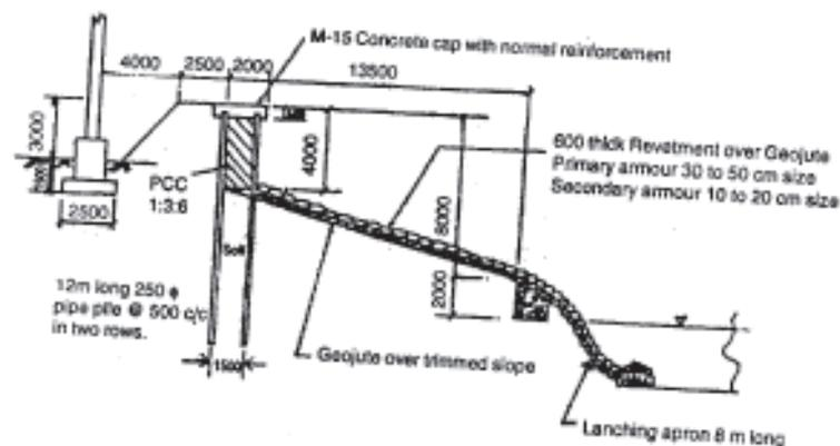
Figure 7 : Geotextile below revetment for river bank erosion in Lakwa, Assam
